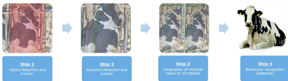
Figure 3. Pipeline for creating timeseries of 3D keypoints.
